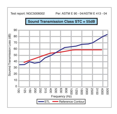
Sound Transmission Loss data for tile floor/ceiling assembly with 32oz. Acoustiblok, STC 55. See illustration and description on previous page for details of the assembly. Unlike other noise barriers, Acoustiblok's performance remains high at the lowest sound frequencies.
